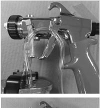
Illustration #2: The original air tube is removed from the spray gun, and the air pressure elbow on the gun body is plugged, using a simple plug made from a 1" piece of air tubing and a sheet metal screw. The tube from the HVCLP is then connected to the air tube fitting on the cup lid cover of the spray gun. This configuration allows for easy attachment and removal of the HVCLP Assembly.
