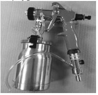
Illustration #1: The HVCLP is connected inline to the hose attachment of the spray gun, between the gun body and the turbine air hose, using the supplied quick disconnect fitting.
