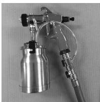
Illustration #3: The spray gun is properly configured with the HVCLP and turbine hose. The lower valve on the turbine hose will regulate the fluid pressure, and then the upper valve on the HVCLP will further regulate the air pressure at the tip. This will allow for higher material flow at lower atomization, resulting in larger particle variation, for a more natural stone look on countertops.
